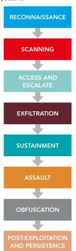
TABLE 6.1: Stages in a cyber-attack and potential countermeasures
